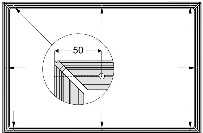
**3** Mount the wall brackets using screws.
