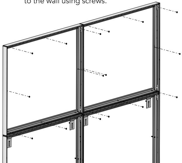
**8** Fasten the frames together (horizontally & vertically) with self drilling screws to prevent gaps.
