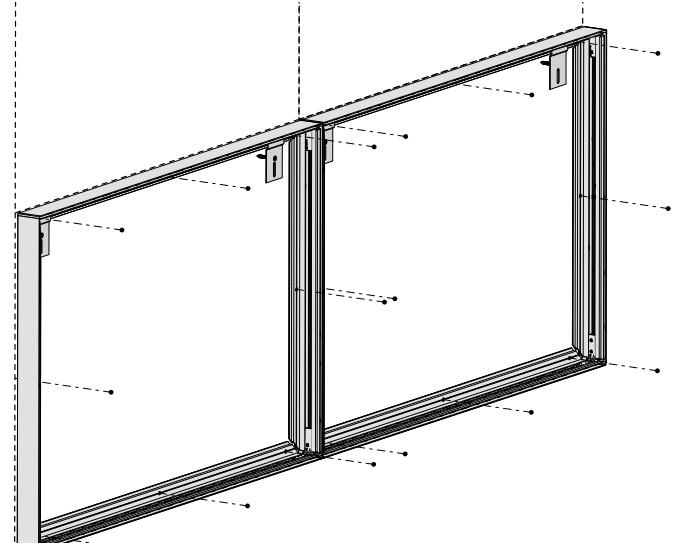
**6** Fasten the frames together vertically with self drilling screws to prevent gaps.
