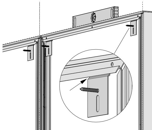
**5** Secure the bottom frames to the wall using screws.
