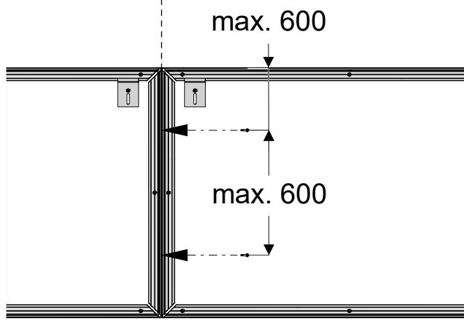
**7** Secure the upper frames to the wall using screws.
