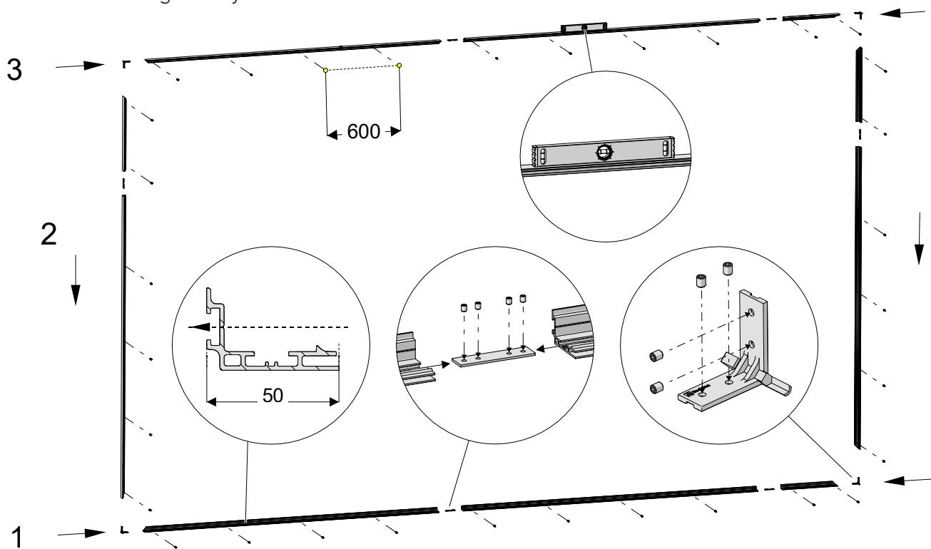
**2** Insert the first absorber. Slide the connectors into the vertical side of the absorber, ensuring a 5 mm air gap between the back of the absorber and the wall, and fix them to the wall.
