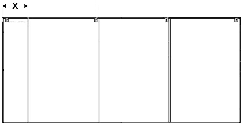
**2** Mount the wall panel on the wall brackets.
