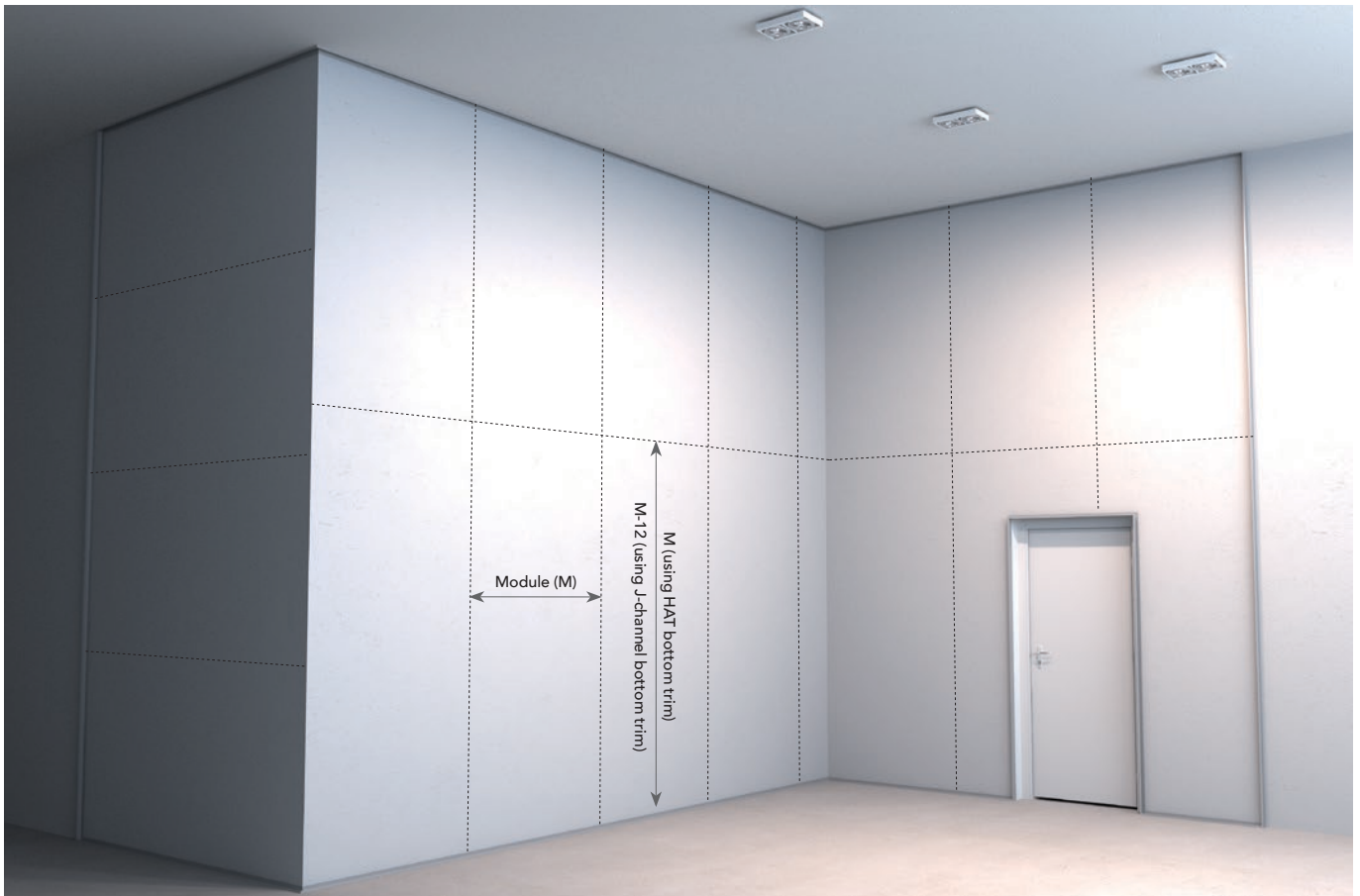
1.1 Mark out all the axes for perimeter trims and intermediate profiles.
