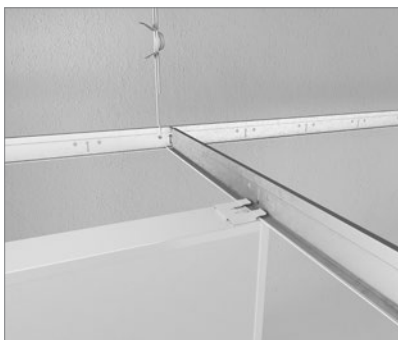
Rockfon Universal Baffle correctly fixed to a Chicago Metallic T24 profile (both connecting tabs clicked on the table of the T24 profile).
